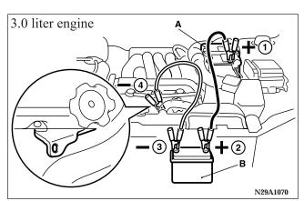
6. Connect one end of the other jumper cable to the negative (-) terminal of the booster battery (B), and the other end to the engine block of the vehicle with the discharged battery (A) at the point farthest from the battery.
